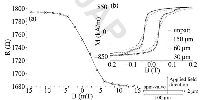
FIG. 1. (a) Hysteresis cycle of the spin-valve sensors used, showing a linear behavior with a magnetoresistance effect of 6.9%. The current applied for the measurement was 0.2 mA. The inset (b) shows hysteresis cycle of the magnetic reference element, for an unpatterned sample and for different patterned sizes. The sample deposited on glass patterned, respectively, with rectangles of 100  $\mu\text{m}$  (150, 60, 30  $\mu\text{m}$ ).
