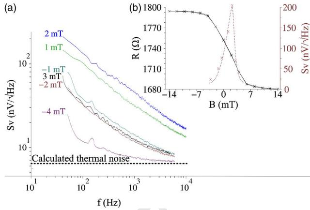
FIG. 2. (Color online) (a) Noise measurement of used sensors, measured at room temperature for a current of 0.2 mA and a resolution bandwidth of 20 Hz. Inset (b) shows the level of low frequency (30 Hz) noise superimposed with the hysteresis curve. Continuous line is a guide for the eyes.
