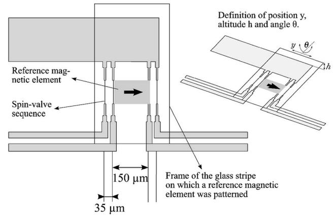
FIG. 3. Design of the spin-valve sensors. The magnetic reference element, of  $100 \times 150 \mu\text{m}^2$  can be seen on top of the spin valves, with an arrow indicating its magnetization direction. In the inset, definition of the coordinates  $y$  (lateral position),  $h$  (altitude), and  $\theta$  (angle). The illustrations correspond to the horizontal geometry of measurement.
