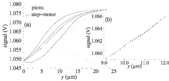
FIG. 5. (a) Experimental scan in the sensitive area (zone where the signal changes fast while the reference element is moved over the sensors), using a piezoelectric actuator and a step motor. The hysteresis opening shown comes from the actuation mechanism. The inset (b) shows in detail the output for a movement by steps of 0.1  $\mu\text{m}$ .
