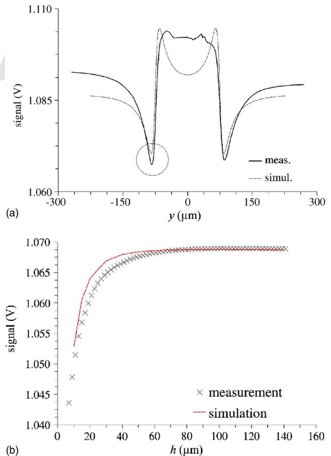
FIG. 4. (Color online) Simulated and measured output. (a) Measurement of the signal of a spin valve when the reference element is passing over it, for a full-range measurement. The circled area corresponds to a zone where the variation of signal is highest signal change with the altitude of the reference element. (b) An approach made in the circled area, where the altitude  $h$  is changed between 5 and 160  $\mu\text{m}$ .
